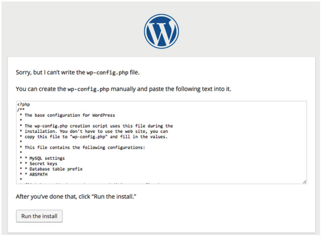
Figure 7-5. Configuration file created by WordPress installation
