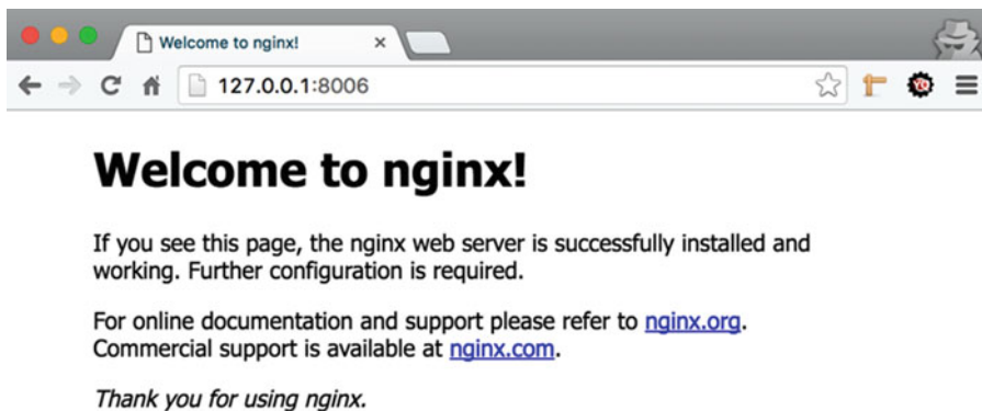
Figure 6-5. Browsing an Nginx website using port forwarding from a host machine
