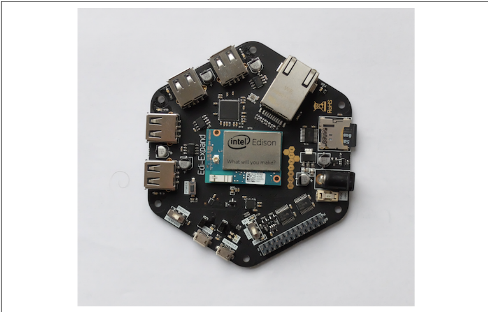
Figure 6-5. The Edison mounted on the Edi-Expand from Tektyte
