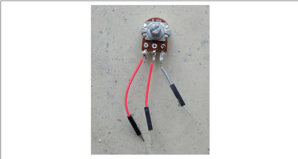
Figure 7-5. A potentiometer with jumper wires soldered onto it
