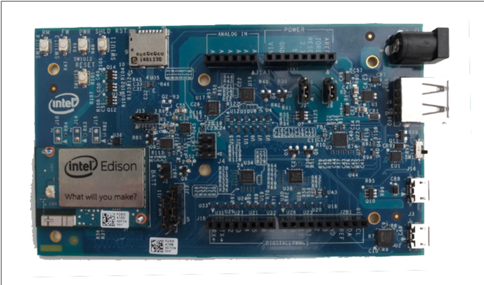
Figure 6-4. The Edison package on an Arduino breakout board
