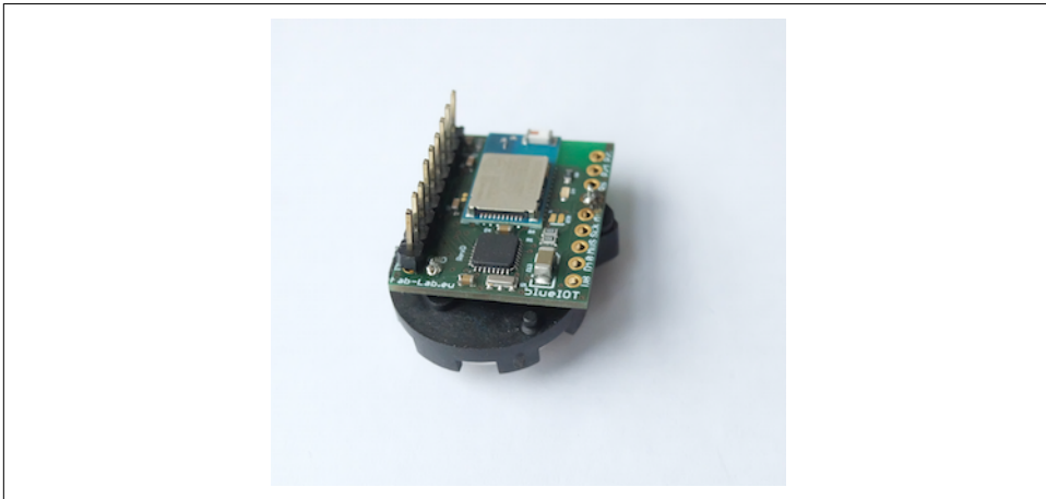
Figure 13-7. BlueIoT board from fab-lab.eu (via tindie.com)
