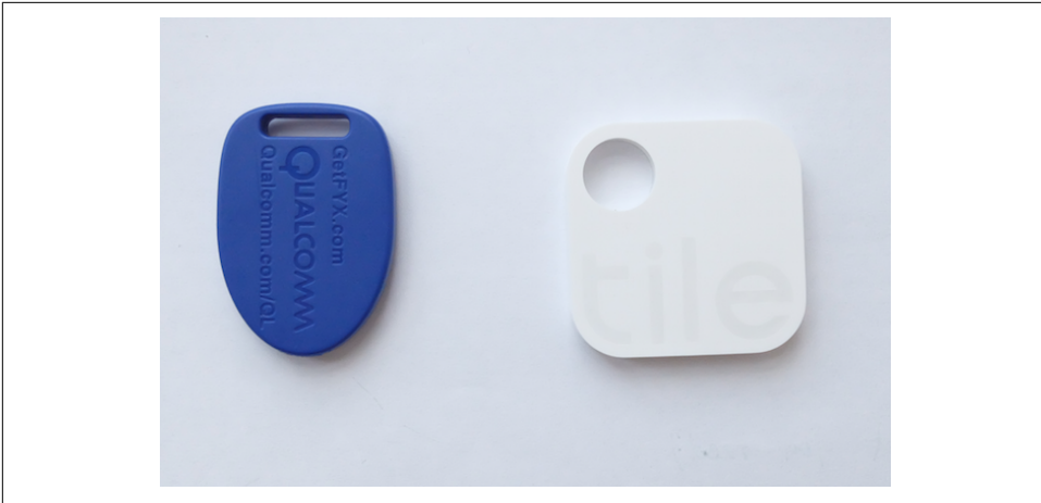
Figure 13-4. The Gimbal (left) and Tile (right) are just two examples of BLE beacons
