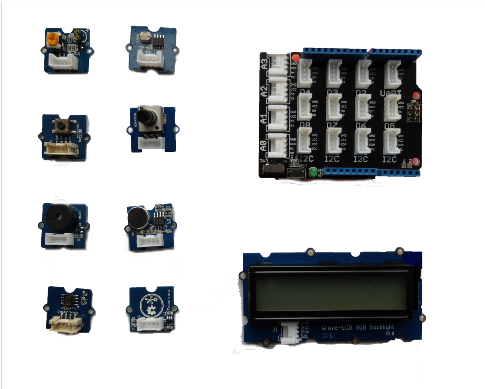
Figure 7-2. The Grove base shield (top right) provides headers to easily connect components (left and bottom)
