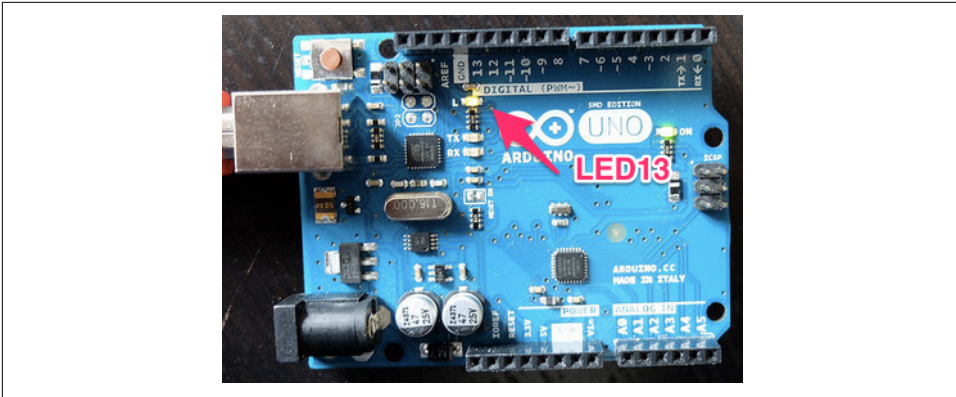
Figure 2-5. The default LED to blink on the Arduino Uno
