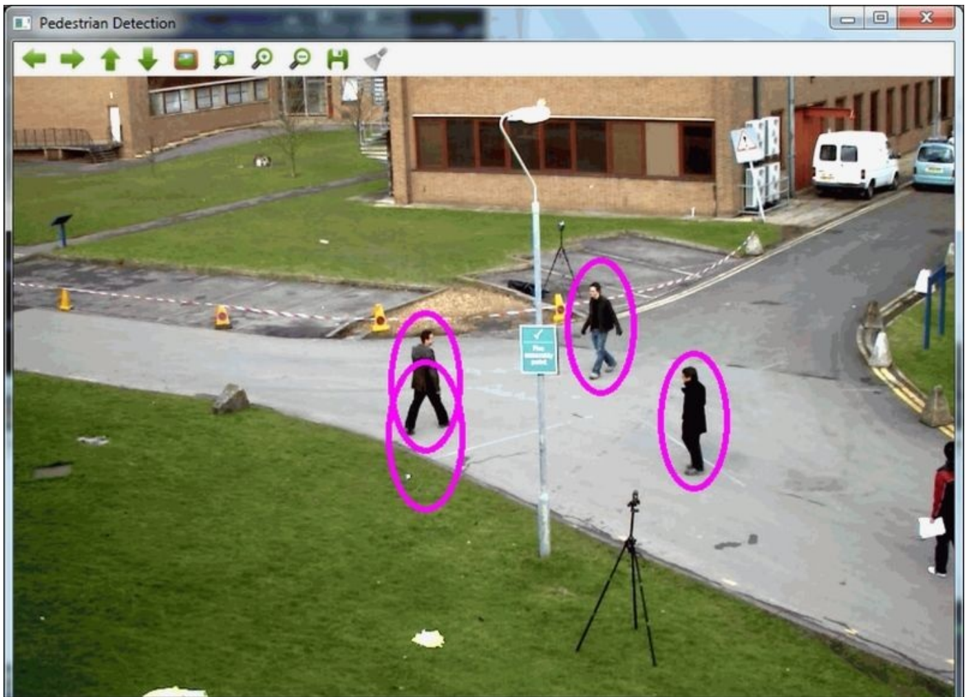
Pedestrian detection using the OpenCV-trained HOG cascade detector
