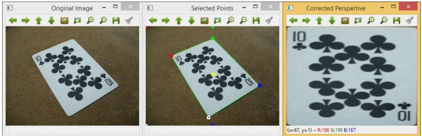
Output of the geometrical transform performed to correct the perspective
