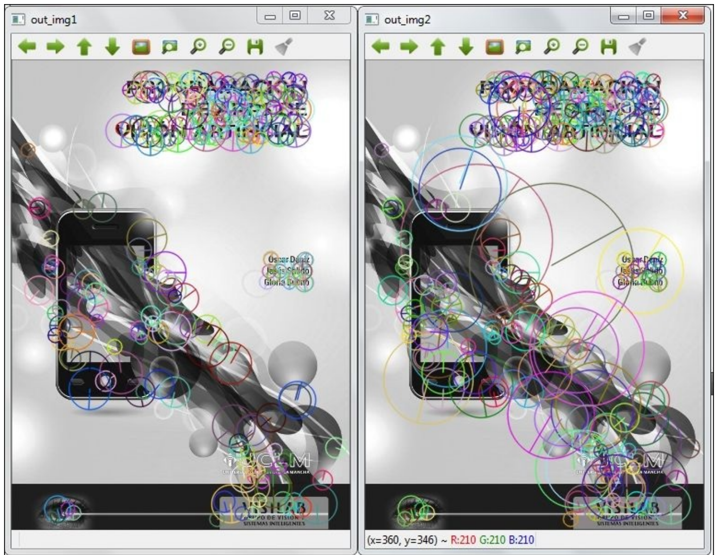
The SURF detector with two Gaussian pyramid octaves (in the left-hand side) and the SURF detector with five Gaussian pyramid octaves (in the right-hand side)
