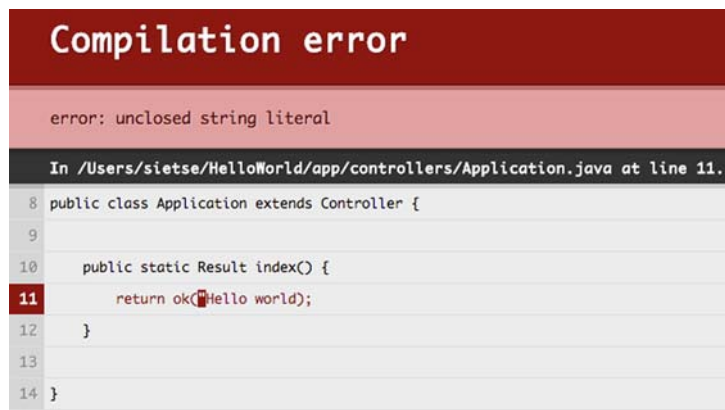
Figure 1.5 Compilation errors are shown in the web browser, with the relevant source code highlighted.
