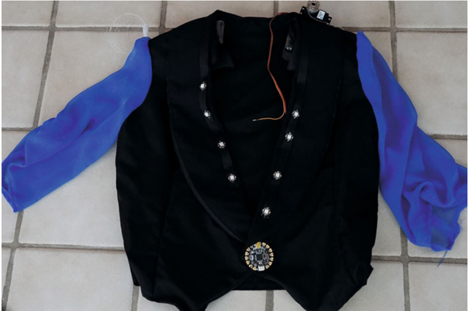
Figure 10-4. The dress jacket showing NeoPixels, Flora, and some of the servo/fishing line attachments
