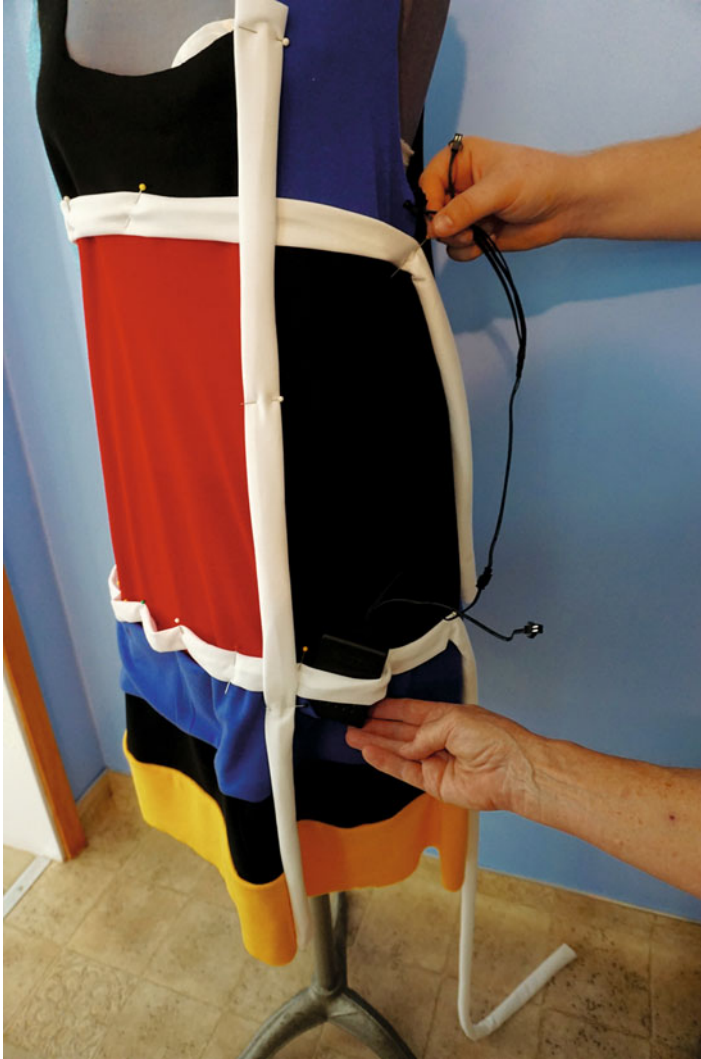
Figure 11-21. Placing the ribbon casings on the dress and experimenting with wire routing (ultimately I routed from the other side)
