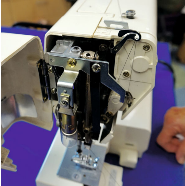
Figure 3-16. The upper thread guide
