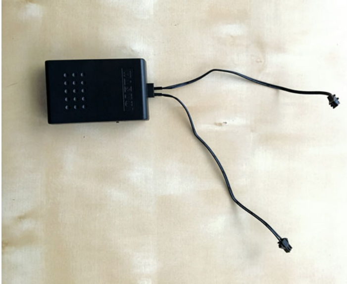
Figure 11-23. Inverter/battery packs and cabling you will need (with two connectors)
