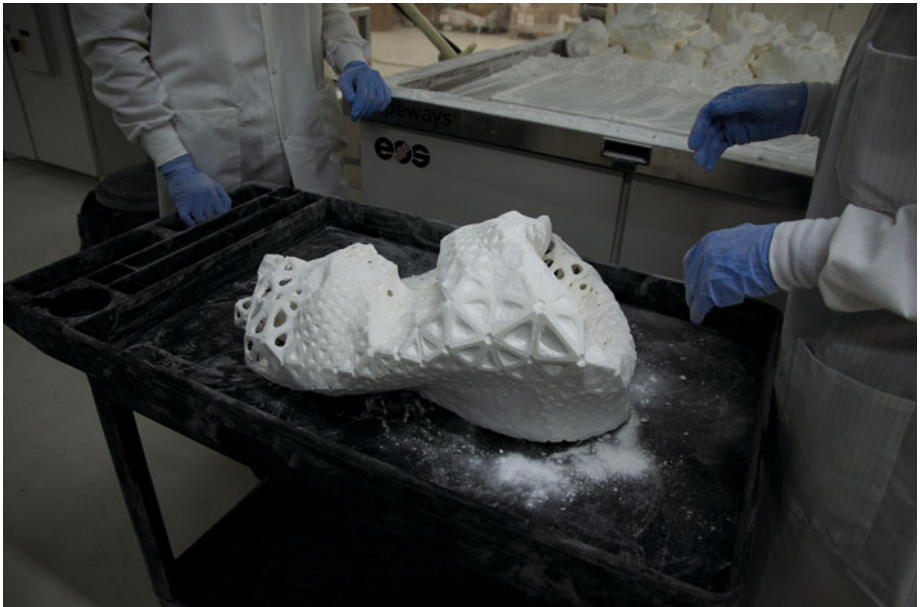
Figure 13-3. The Kinematics Dress 1 before all the excess powder was removed. Image courtesy of Nervous System.
