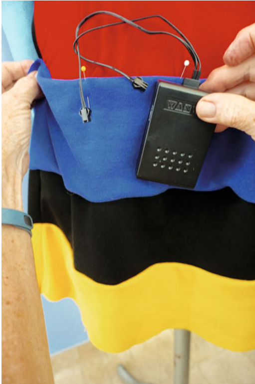
Figure 11-18. Checking that the battery pack/inverter will fit into its pocket
