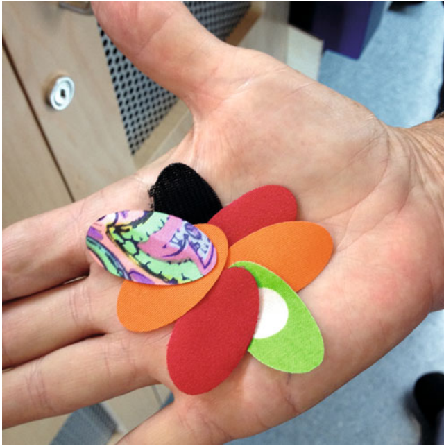
Figure 12-2. Test pieces of various fabrics after laser cutting (the green one was cut in the setup of Figure 12-1)
