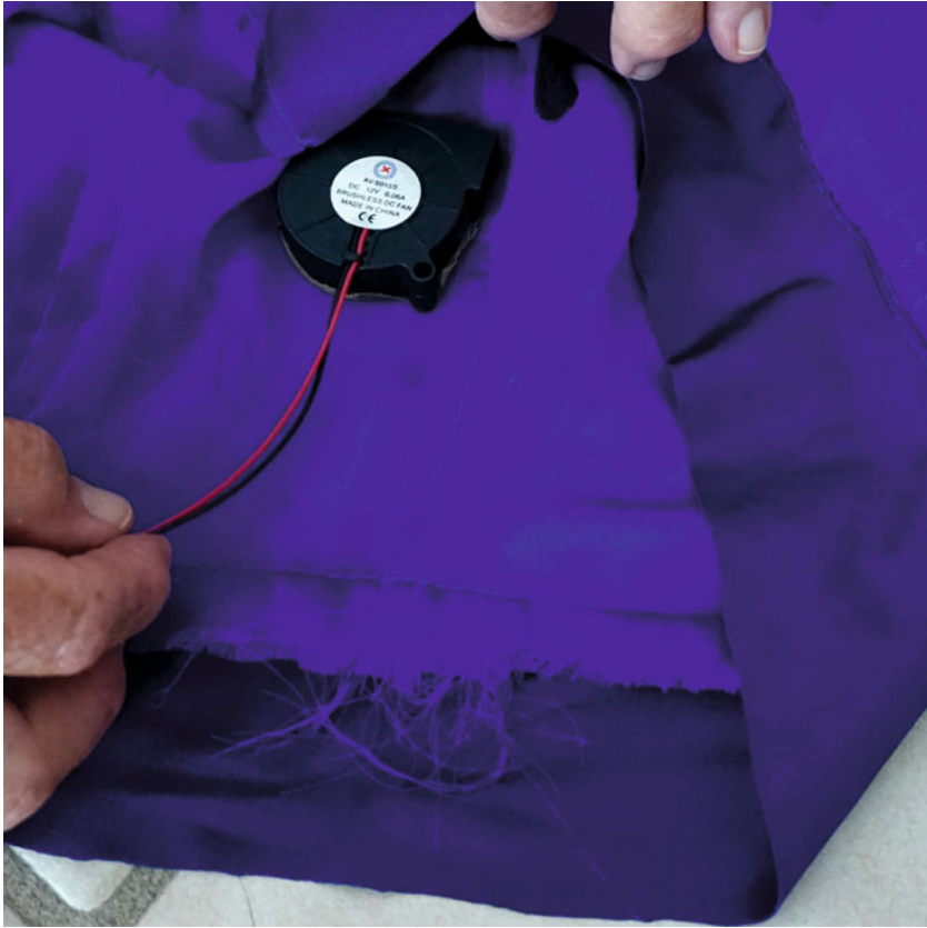
Figure 10-10. The fan being slipped out of its pocket
