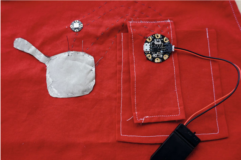
Figure 7-13. Layout of the electronics placket, battery holder, Gemma, NeoPixel, and conductive hand stitching
