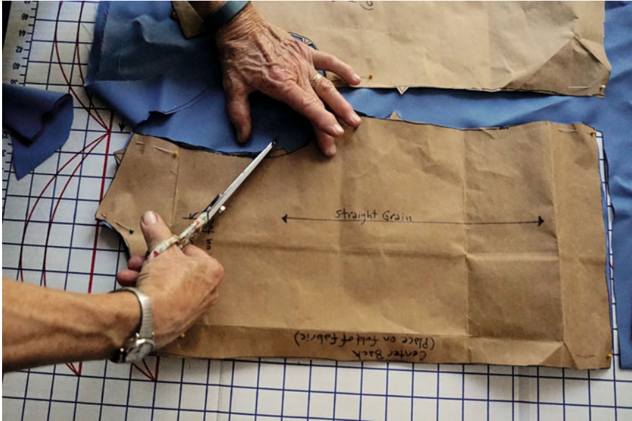
Figure 4-7. Leaning on the fabric to cut a notch
