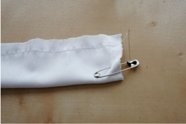
Figure 11-19. Creating the EL ribbon casing, with a pin to turn it right-side out
