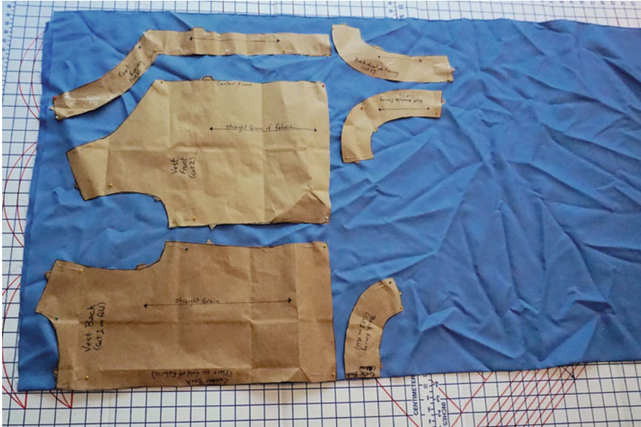
Figure 4-5. The vest pattern (on a fabric without a nap) pinned on fabric on a cutting board. The fold is at the bottom, selvage on top.
