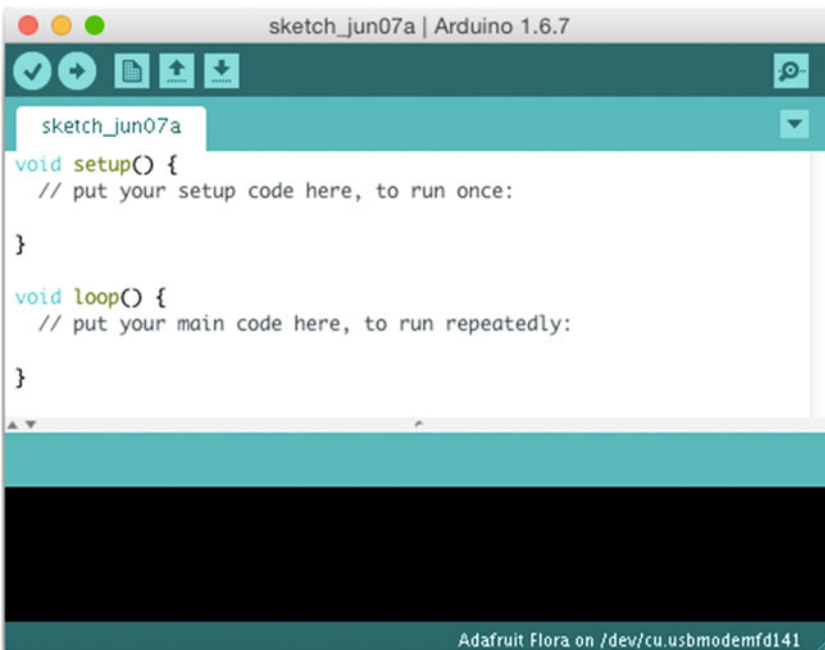
Figure 6-2. The Arduino IDE default sketch. Note that it tells you on the bottom right what type board it thinks that you are using.
