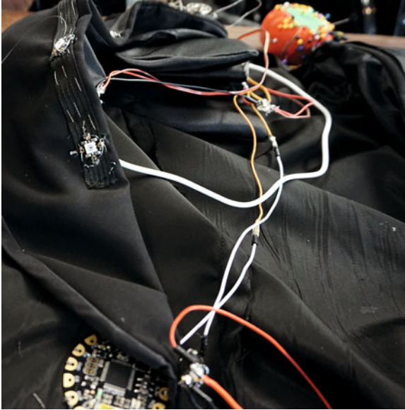
Figure 10-1. Unplanned wiring gets out of hand
