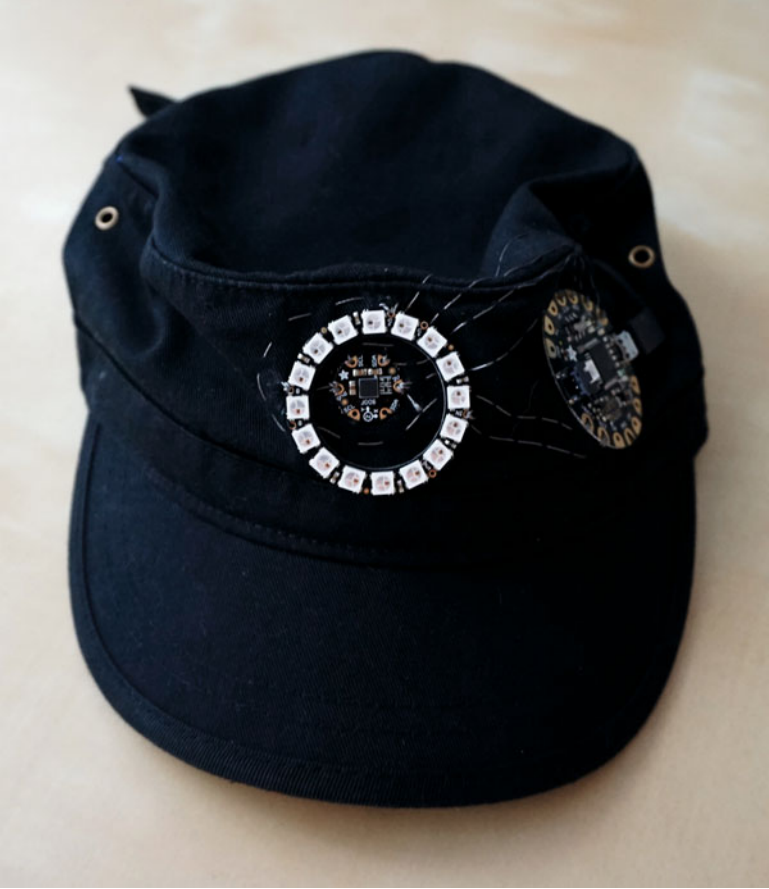
Figure 11-1. The yes-no hat (with NeoPixel ring off)
