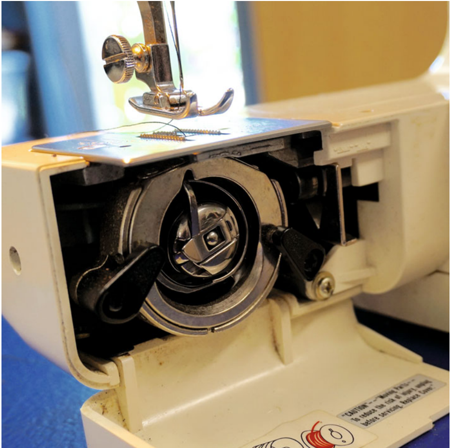
Figure 3-19. Bobbin placement on front, near the bottom, on a differently designed machine
