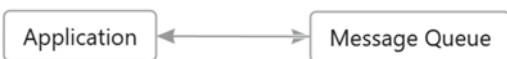
Figure 5-3. An example of a relationship that is not unidirectional, delineated by bidirectional edges
