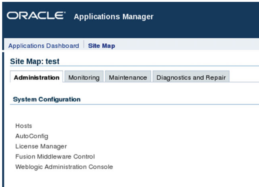
Figure 8-4. EBS 12.2: OAM AutoConfig administration
