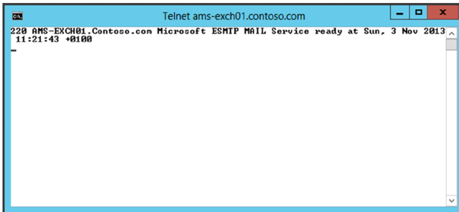
Figure 9-2. Using the Telnet client to check if server is accepting connections—in this example, the SMTP Transport service on port 25
