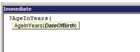
Figure 1-9. Whenever you type the opening parenthesis after any procedure name in the VBA environment, all arguments required by the code procedure will be shown to you
