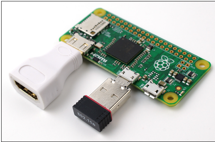
FIGURE 2-7: A Pi Zero with Wi-Fi dongle (right) and mini-HDMI to HDMI adapter (left)
