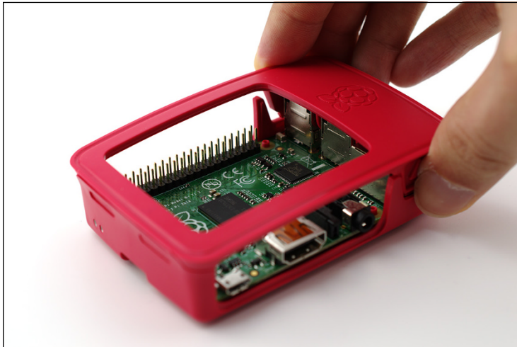
FIGURE 16-3: Assembling the top of the case
