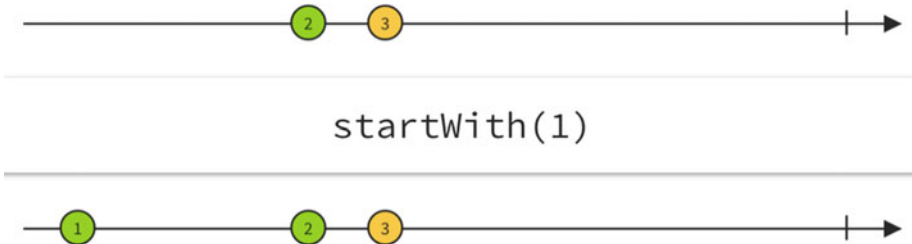
Figure 2-11. A marble diagram of the startWith operator
