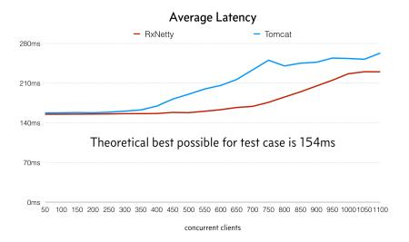
Despite averages not being very valuable (as opposed to percentiles), this graph shows how both have similar latency with little load, but diverge significantly as load increases. Netty is able to better utilize the machine until higher load with less impact on latency:
