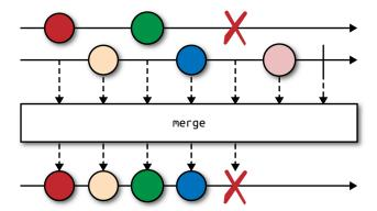
The merge() operator is used extensively when you want to treat multiple sources of events of the same type as a single source.<sup>4</sup> Also, if you have just two Observables you want to merge(), you can use obs1.mergeWith(obs2) instance method.
