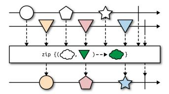
The zip() and zipWith() operators are equivalent. We use the former when we want to fluently compose one stream with another, like so: s1.zipWith(s2, ...). But when we have more than two streams to compose, static zip() on Observable can take up to nine streams:
