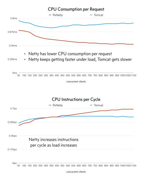
Netty CPU consumption remains mostly flat through increasing load and actually becomes slightly more efficient as the load is maxed out, as opposed to Tomcat, which becomes less efficient.
