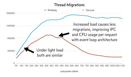
Note how the lines diverge as load increases. These are the thread migrations. The most interesting thing I learned was that the Netty application actually becomes more efficient as it is put under load and the threads become "hot" and stick to a CPU core. Tomcat, on the other hand, has a separate thread per request and thus cannot gain this benefit and retains higher thread migrations due to each thread needing to be scheduled for every request.
