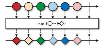
The map() operator takes a function that can change the shape of input event from circle to square. This transformation is applied to each item flowing through it.
