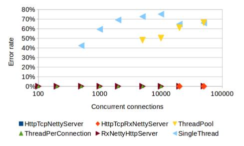
Errors, as reported by the wrk load test tool are nonexistent to marginal for all of the implementations except SingleThread and ThreadPool. This is an interesting trade-off: ThreadPool always responds as soon as possible, much faster than competitors. However, it is also very eager to reject requests immediately when it is being overwhelmed. Of course, you can implement a similar mechanism on top of a reactive implementation with Netty/RxJava.
