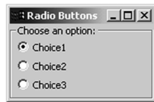
Figure 3.9 With a RadioGroupFieldEditor object, you can display a set of radio buttons without creating individual Button objects.
