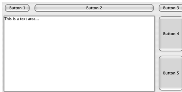
Figure 6.6 A more advanced GridLayout . The text area covers two columns and two rows. All the other controls are contained in one cell each.
