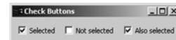
Figure 3.7 Check buttons let the user select zero or more options from a group.
