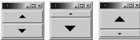
Figure 3.12 SashForms allow the user to specify the relative sizes of the Composite 's children.
