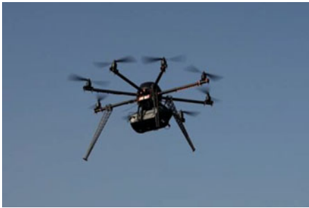
Figure 8-2. An Interspect UAS B 3.1 Photogrammetry Platform, one of the new generation of military surveillance drones
