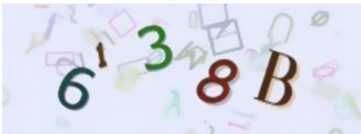
Figure 7-1. A CAPTCHA , which is text that is easy for a human to recognize but hard for a computer
