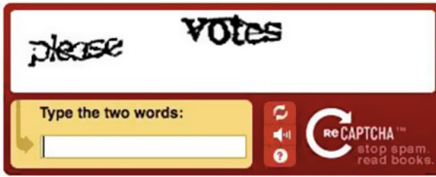
Figure 7-2. Example of a ReCAPTCHA, the extension of the CAPTCHA into a successful form of human computation used to help process texts for optical character recognition (Used with permission)
