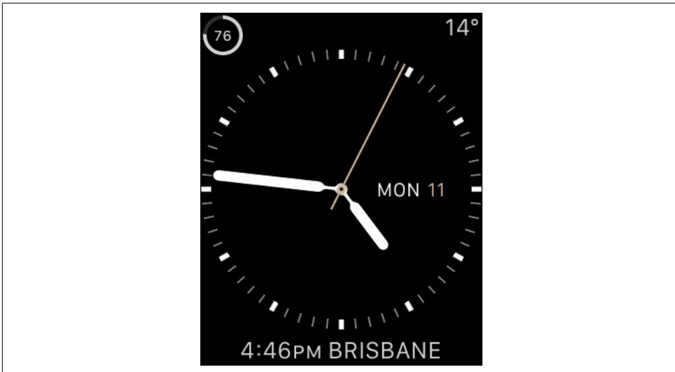
Figure 5-1. Several complications on the watch face (except for the watch dial and hands, everything in this image is a complication)
