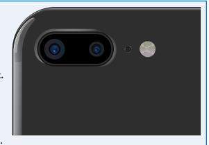
The iPhone 7 Plus has a dual-camera module on the back rather than a single-camera module, as the other models have. One camera as a 28mm wide-angle lens, while the other has a 56mm telephoto lens to provide optical zoom, which gives higher image quality than the digital zoom provided by enlarging pixels via software.
