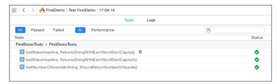
When you hover over one of the tests with the mouse pointer, a circle with an arrow to the right appears. If you click on the arrow, Xcode opens the test in the editor.
