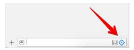
If this button is clicked on, only the failing tests are shown in the list.
