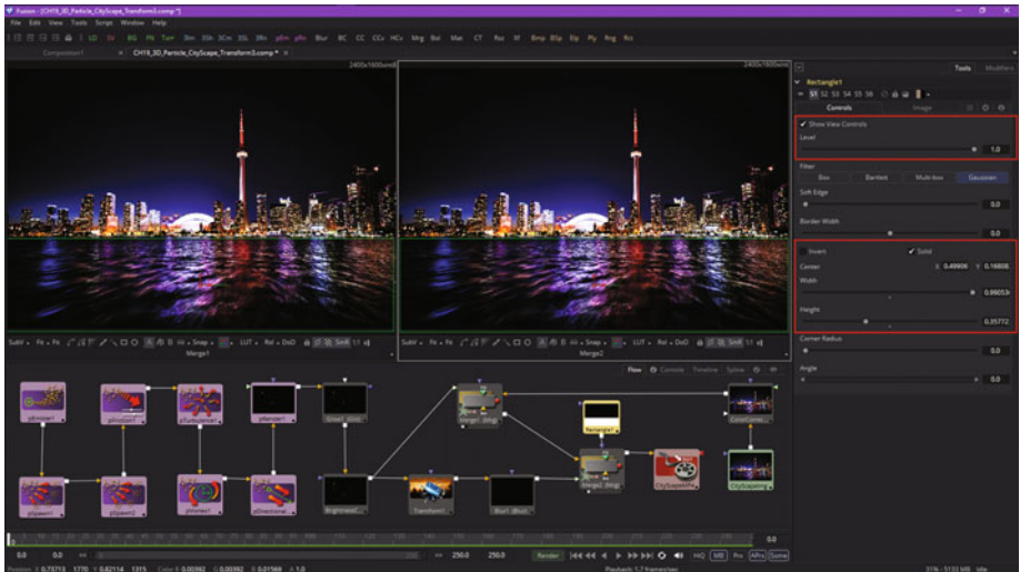
Figure 19-20. Set the Rectangle1 mask widget so that it will cover the water areas
