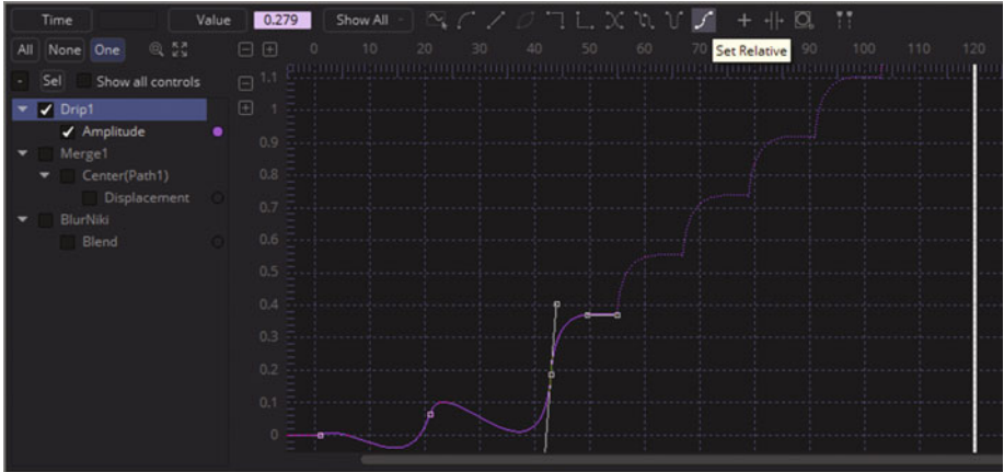
Figure 10-22. Click the Set Relative icon to loop and offset curve segment
