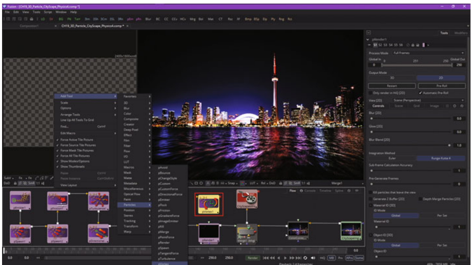
Figure 19-7. Add a pVortex node tile to your particle physics simulation node processing pipeline
