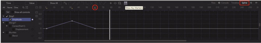
Figure 10-1. Click the Spline tab, then select the Amplitude control
