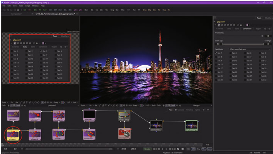
Figure 19-12. Eliminate the circuitous set reference in pSpawn1 to eliminate the problem
