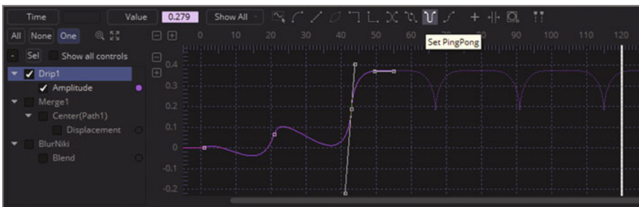
Figure 10-21. Click the Set PingPong icon to loop and mirror curve segment
