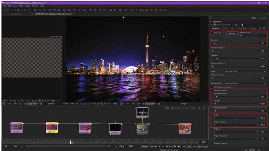
Figure 18-12. Set pSpawn parameters for Number, Angle, and Velocity
