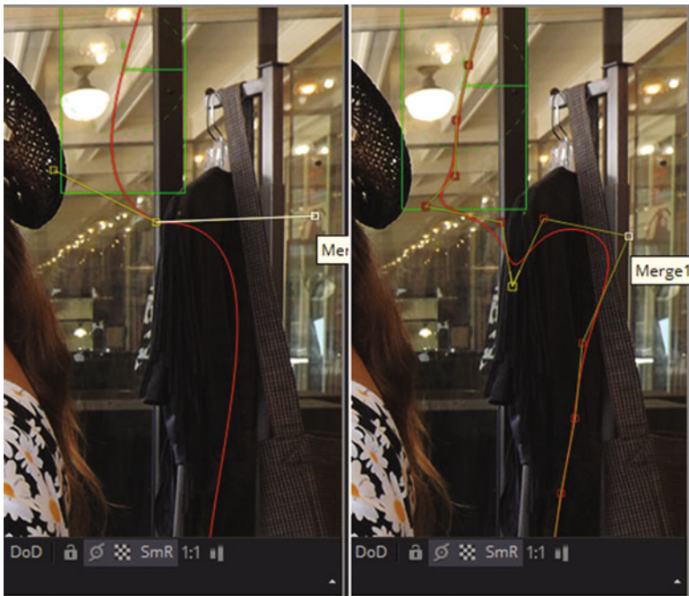
Figure 11-2. Bézier curve converted to B-spline
