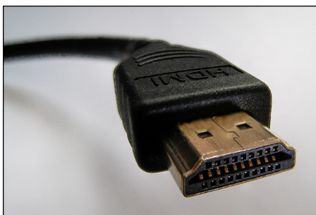
FIGURE 1-13: HDMI has largely supplanted the old VGA and DVI-D video adapters.
