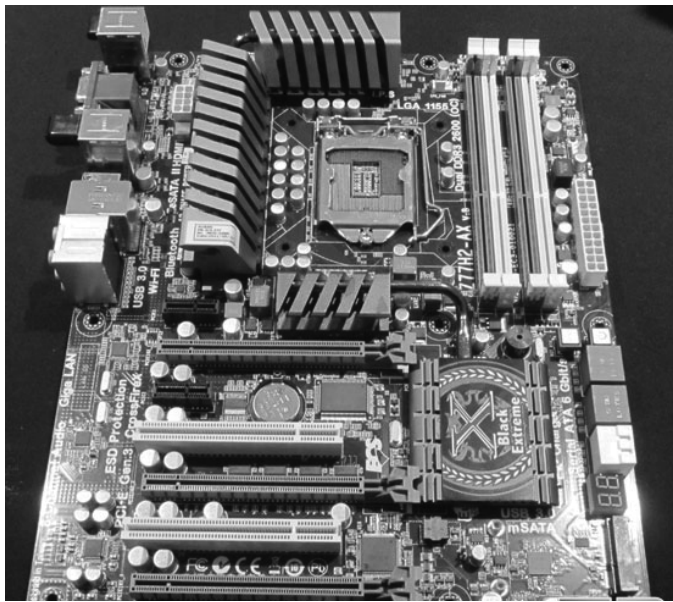
FIGURE 34.9 Slots on a computer motherboard.
