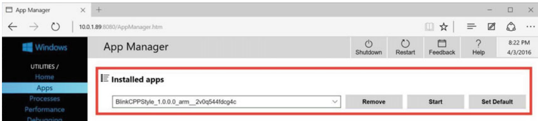
Figure 5-14. Starting an application on the device
