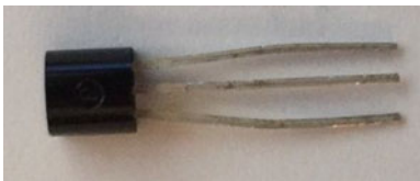
Figure 15-12. TMP36 temperature sensor
