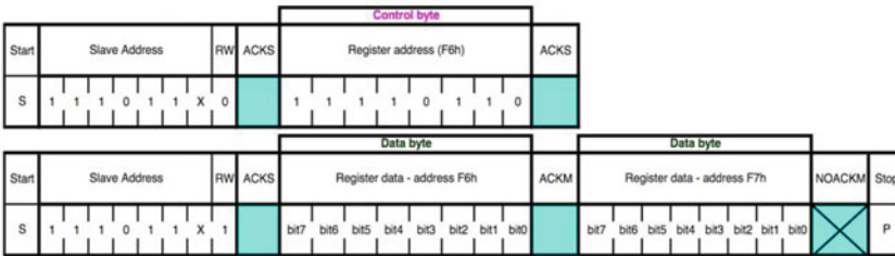
Figure 8: I 2 C multiple byte read
