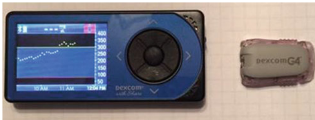
Figure 1-2. Dexcom continuous glucose monitor with sensor
