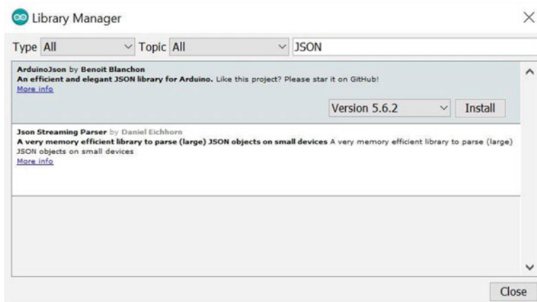
Figure 15-19. Installing the ArduinoJSON Library: Arduino IDE
