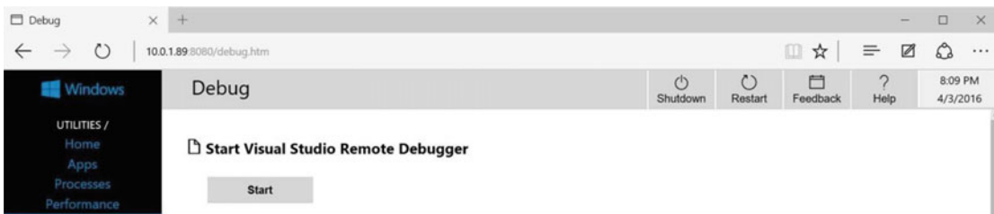
Figure 6-9. Turning on the remote debugger
