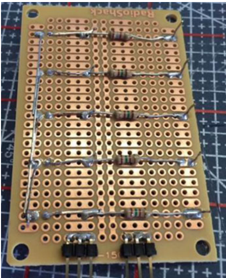
Figure 14-13. Completed protoboard (LED circuit board)
