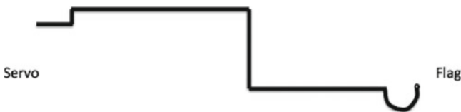
Figure 14-14. Forming the servo rod/cable
