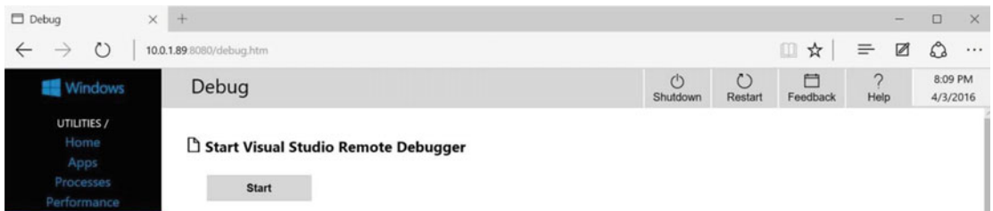
Figure 5-13. Turning on the Remote Debugger
