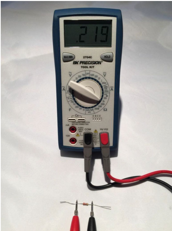
Figure 8-11. Measuring resistance of a resistor
