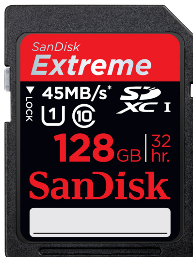
Figure 1-6: A 128GB SD card. MicroSD cards slip in to holders shaped like an SD card.
