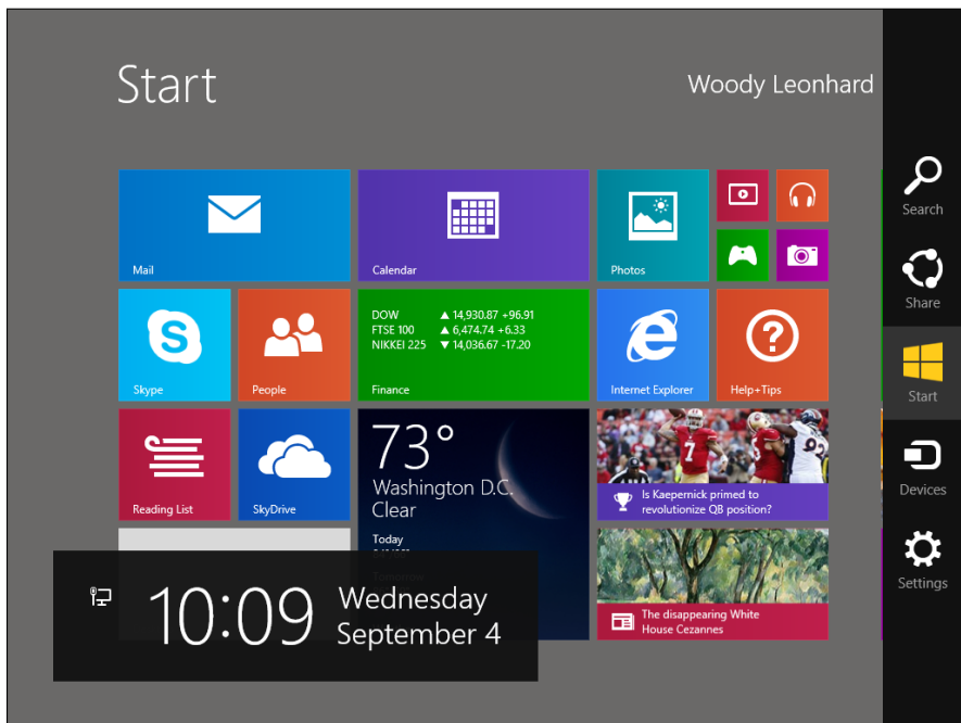
Figure 3-1: The Charms bar on the right side of the screen.
