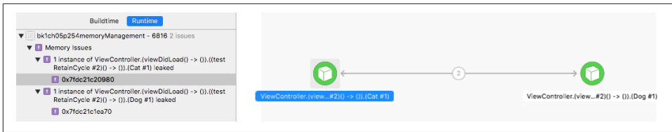
Figure 9-18. The memory graph displays a leak
