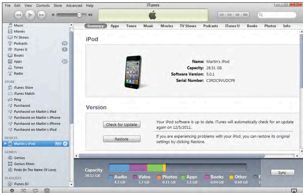
Figure 25–3. Connecting your iPod touch and clicking the Restore button in the Summary screen
