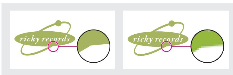
Logo drawn as vector art (left), and rasterized as bitmap art (right).
