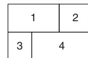
Figure 12.6 Map in which different regions are to be assigned colours so that the number of colours is minimum and no two adjacent regions have same colour
