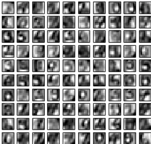
Figure 6.14 A graphical representation of the weights between the hidden and visible units in our RBM. Each square represents a single hidden unit, and the 64 grayscale values within represent the weights from that hidden value to all the visible units. In a sense this dictates how well that hidden variable is able to recognize images like the one presented.
