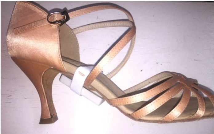
Figure 17-14. A simple, but efficient way to attach the sensor to a dancer's heel
