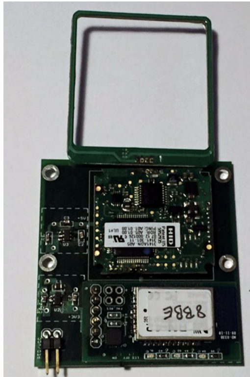
Figure 17-2. A wireless proximity card detector such as this MFi accessory uses standard Bluetooth for communications with the iOS device
