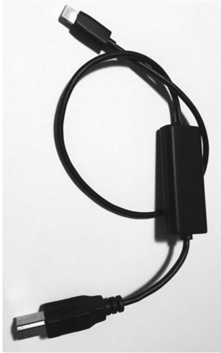
Figure 17-1. This sports accessory that connects a rowing machine to your iPhone uses the Lightning connector to make a physical high-speed connection
