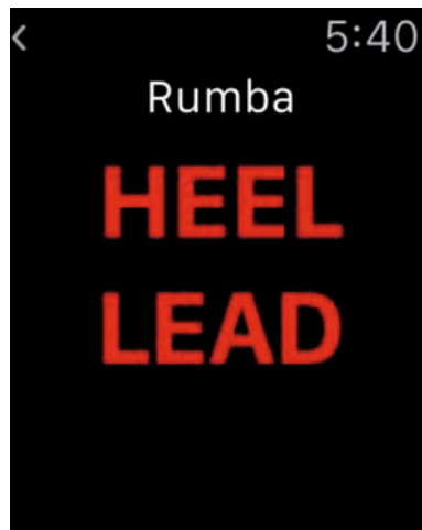
Figure 17-12. If the angle of the sensor on the shoe is not correct for the dance style selected, in addition to an audio-visual indication, the Watch vibrates to let the dancer know of her error
