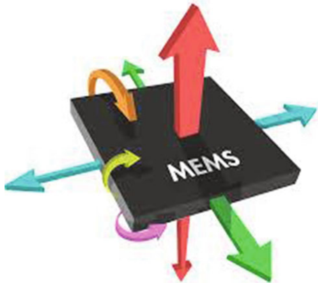
Figure 13-8. Readily available devices can measure movement and orientation in each of three axes and provide that information over standardized communications ports
