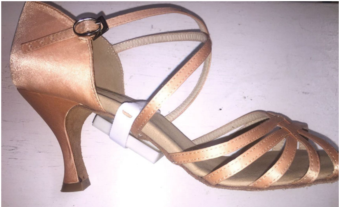
Figure 13-10. Using nothing more than a 3D-printed plastic PCB carrier and a strip of Velcro, the author was able to test the sensor system on an actual dance floor
