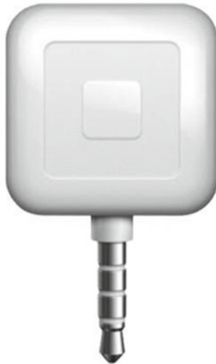
Figure 1-14. The Square credit card reader, one of the earliest iPhone accessories, used the headphone jack instead of the 30-pin dock connector, making it cross-platform compatible
