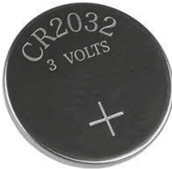
Figure 13-19. Designed to work with standard coin cell batteries, BTLE provides a low-power solution for circuitry that needs to only transmit small amounts of information infrequently
