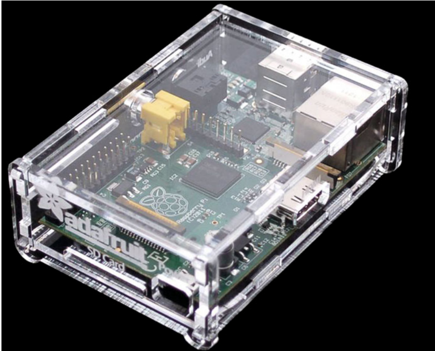
Figure 9-7. For those embedded systems where cost is a key concern, off-the-shelf modules such as this Raspberry Pi may be all you need
