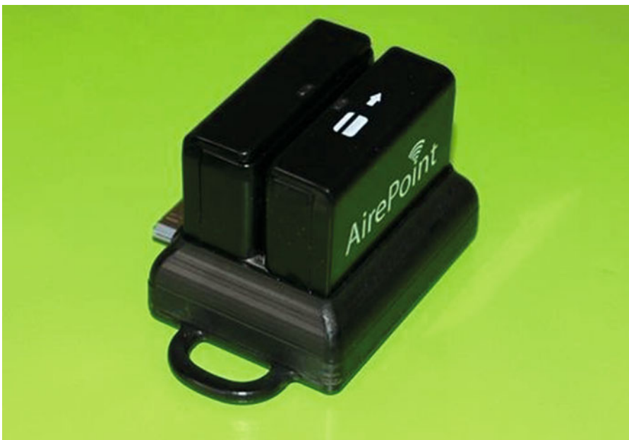
Figure 13-1. The author designed, manufactured, and sold one of the first commercially available credit card swipe accessories for the iPhone in late 2009
