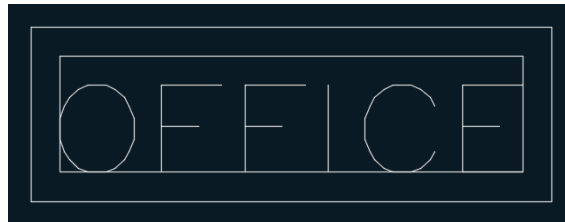
FIGURE 10.4 Making single-line text fit within a predefined space
