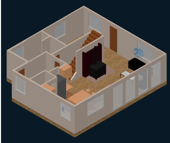
FIGURE 18.5 Using the realistic visual style to display materials' texture maps
