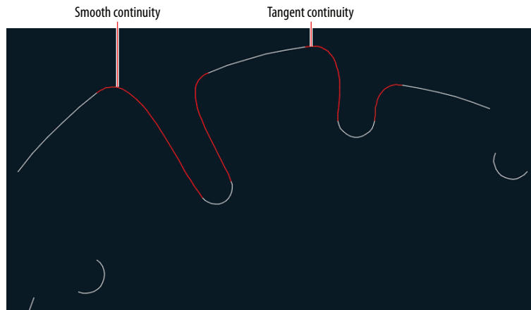
FIGURE 5.20 Blending between arcs with different types of continuity
