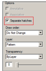
FIGURE 8.15 Separating multiple bounded areas into multiple hatch objects
