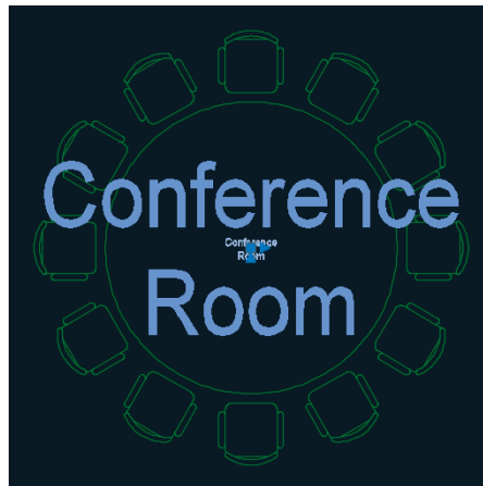
FIGURE 13.5 Annotative text shown in two scales
