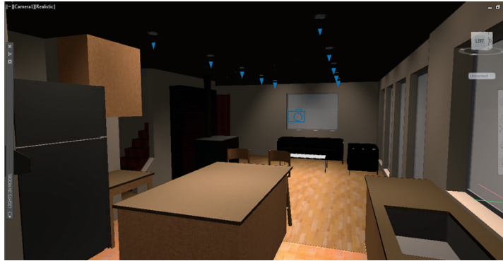
FIGURE 18.12 Selected spotlights reveal light coverage as seen in the camera view.
