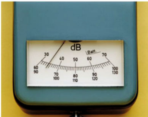
Figure 5-11. A meter measuring signal strength in dB
