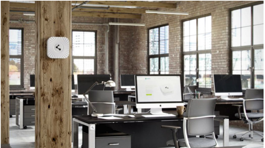
Figure 7-15. Kontakt.io cloud beacon provides a management gateway between its Bluetooth beacons and the ability to monitor and manage via Wi-Fi
