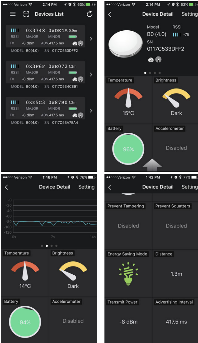
Figure 9-21. The Device List and Detail Screens of the Sensoro app is where individual beacon parameters can be set interactively
