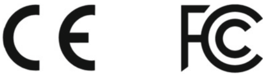
Figure 6-3. The CE Mark and FCC logo indicates compliance with mandatory standards for products to ship in Europe and the United States, respectively
