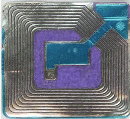
Figure 18-2. The under side of an RFID tag exposing the metallic antenna
