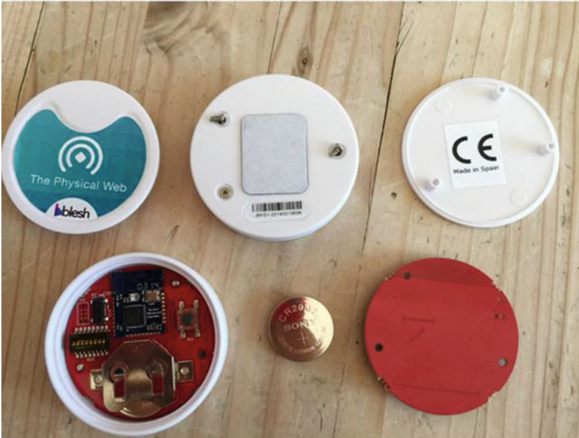
Figure 5-28. Inside a Blesh Physical Web beacon
