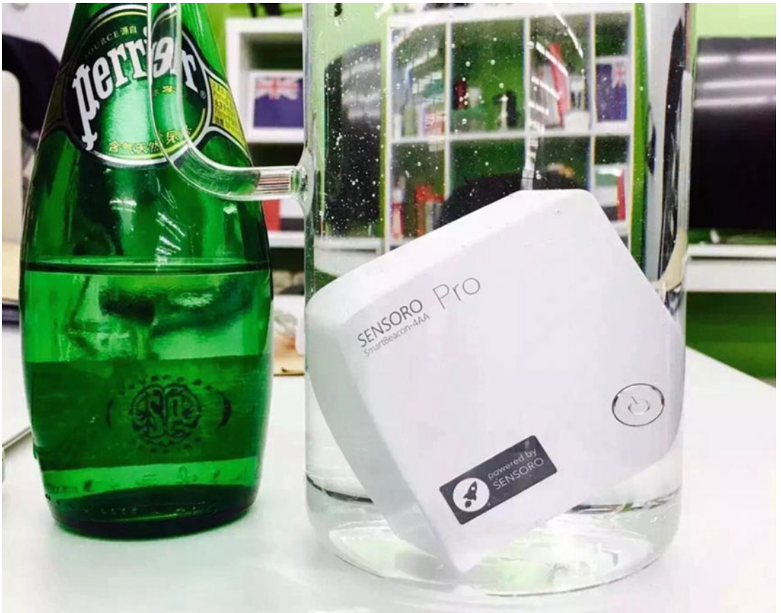
Figure 7-5. The Sensoro Pro beacon is designed to the IP67 standard, being waterproof and dustproof
