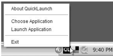
Figure 3-2. QuickLaunch adds a program launcher icon to the system tray.
