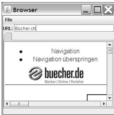
Figure 8-2. Because of the if statement, you can now specify addresses with or without http:// .
