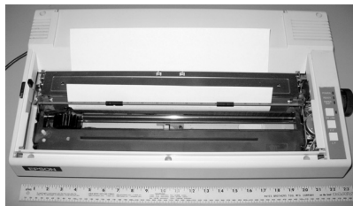
Wide-carriage dot matrix printer. Courtesy: Dale Mahalko (This file is licensed under the Creative Commons Attribution-Share Alike 3.0 Unported license; http://creativecommons.org/licenses/by-sa/3.0/deed.en )
