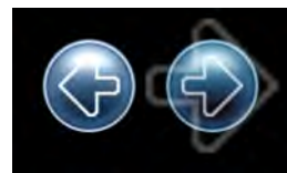
Figure 6.3 The button is constructed from two bitmap images: a background (blue circle) and icon (arrow). When the button is pressed, a ghost of its icon expands and fades.
