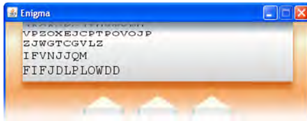
Figure 9.9 Each line of our Paper node is scaled to create the optical effect of a surface curving away, to accompany the shading of the background Rectangle .
