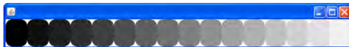
Figure 4.8 Elements inside a Flow are lined up in rows or columns, wrapping when necessary.
