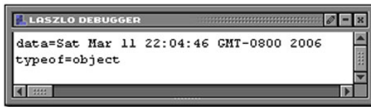
Figure 3.10 The default type of a JavaScript expression is that of a value returned from a JavaScript operation.
