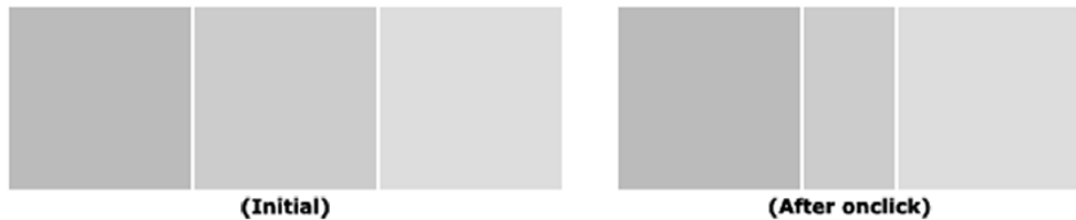
Figure 6.2 Changing the width of a child view participating in a layout results in the layout algorithm being executed.
