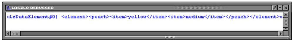
Figure 11.7 The valueToElement method converts JavaScript objects into equivalent XML data structures. It suffers from the limitation of using a default node name ( item ).
