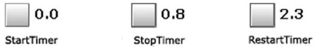
Figure 9.2 The event handler associated with onclick events is dynamically changed. The first time the button is clicked, it starts the timer. The second click stops the timer. This switching of event handlers allows the timer to be repeatedly started and stopped without losing its count.
