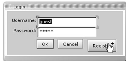
Figure 9.4 LzCursor is used to change the mouse cursor to the pointing hand when over the Register button. The cursor has a “+” in the upper-right corner to indicate that a new user can be added through a Registration window.
