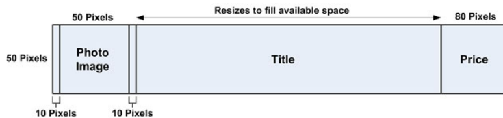
Figure 10.13 High-fidelity wireframe describing the physical layout of each item in the Product List window
