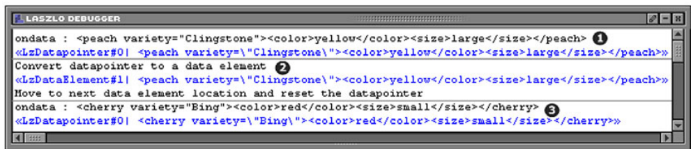
Figure 11.13 A data pointer can be used to retrieve an instance of the data node to which it points, and a data node can be used to set a data pointer.
