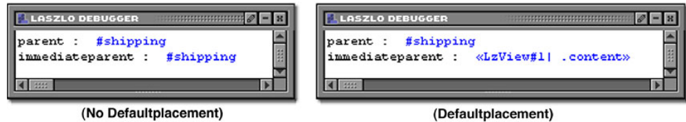
Figure 7.7 This debugger output shows that the text message is the child of the class instance shipping and not of the view content. Both parent and immediateparent have the value shipping.
