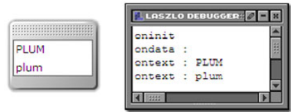
Figure 10.5 The intended output here is a matching pair of uppercase names. However, the ondata change to uppercase is overwritten by the text instantiation. The timing sequence for the instantiation of the text object appears in the debug window.
