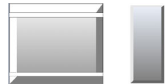
Figure 14.12 The three parts comprising the scrollbar's handle are shown enlarged and out of scale on the left and together as a unit in scale on the right. The top and bottom sections have a height of one pixel. The light lines mark vertical pixels.
