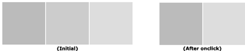
Figure 6.3 Changing the visibility of a child view participating in a layout results in the layout being executed.
