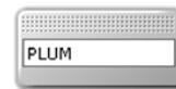
Figure 10.6 The applyData method provides a means to preprocess XML data elements. In this example, the input field is converted to uppercase.
