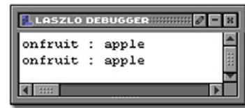
Figure 3.15 Attribute event handling occurs when an attribute's value is updated with the setAttribute method. The updated value can be accessed either through an argument or through the object's attribute itself.
