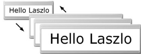
Figure 1.3 The pulsating “Hello Laszlo” example, shown in listing 1.1, uses constraints to create a relationship between the size of the text and the size of the window.
