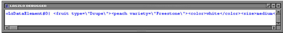
Figure 11.8 The stringToLzData method converts a string into an XML data structure. There is no limit to the length of the string, so an XML structure of arbitrary complexity can be produced.
