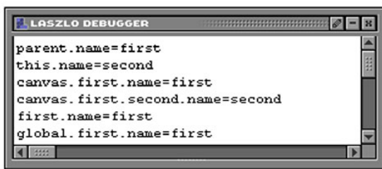
Figure 3.4 Using relative, absolute and top-level references
