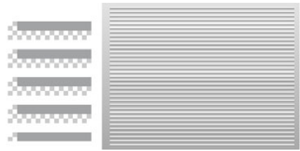
Figure 14.13 The gripper is an alternating sequence of white and gray bars on a transparent background, represented here with a checkerboard. The image on the right demonstrates the visual effect of a gradient against a pattern.
