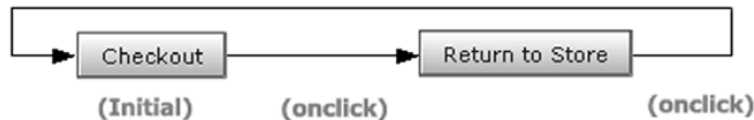
Figure 5.13 The button is initially in the main state, displaying a Checkout label. After the user clicks the button to generate an onclick event, the main state is removed, and the Checkout state is applied. A subsequent click of the button completes the cycle by updating the button label to Checkout, removing the Checkout state, and reapplying the main state.
