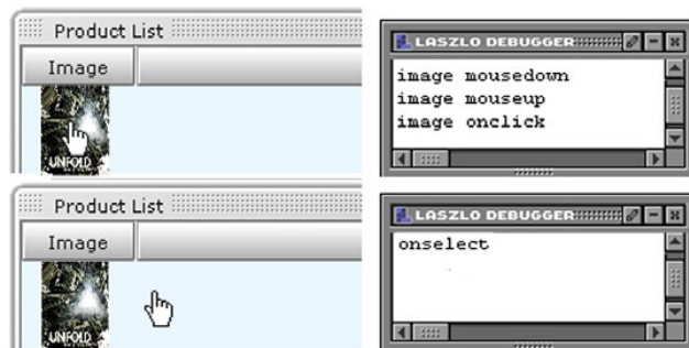
Figure 10.16 The top image illustrates how the mouse events are different, depending on where the mouse selection occurs. Any selections that occur in the image area generate mouse events instead of onselect events.
