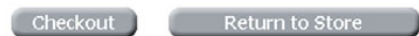
Figure 13.6 A stretchable button is created from three parts. This allows a single button class to be used with a variable-length label to produce buttons that have a consistent appearance.
