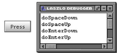
Figure 7.2 When the doesenter attribute is set, pressing and releasing the Enter key or spacebar initiates the appropriate default processing for that key. Pressing the button shown does not cause any of these methods to be called.
