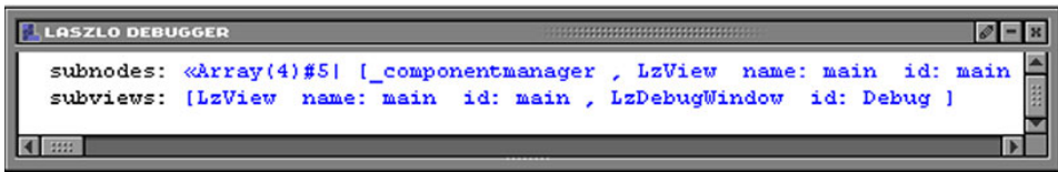
Figure 4.1 Nodes and views are maintained within their respective parent-child hierarchies. These hierarchies are traversed through the subnodes array for nodes and through the subviews array for views. Since the debug window is currently displayed, it appears in the subviews array.
