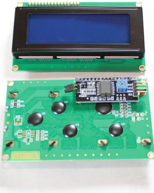
Figure 5-13. Photo of the LCD character display and backpack mounted on the rear
