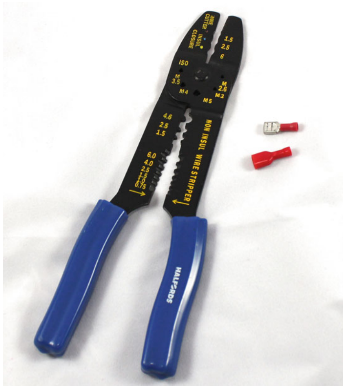
Figure 3-23. Crimp tool with female blade connectors
