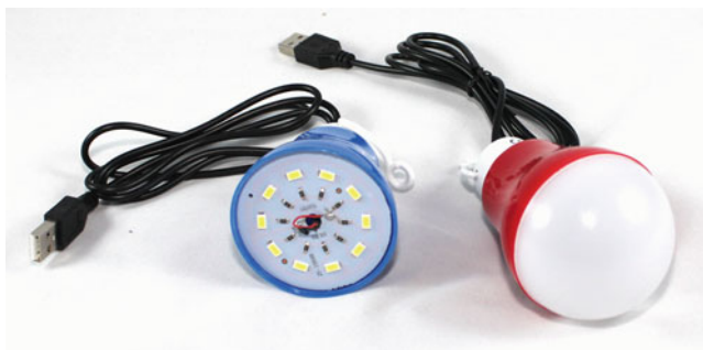
Figure 4-17. LED light with and without the top removed
