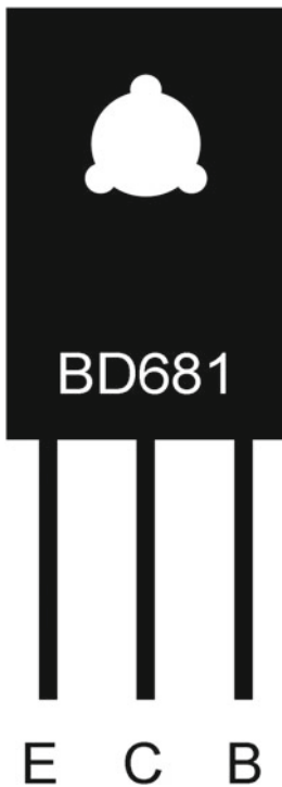
Figure 4-20. BD681 Darlington Transistor pinout
