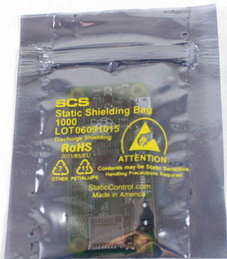
Figure 1-10. Warning symbol for a static-sensitive component
