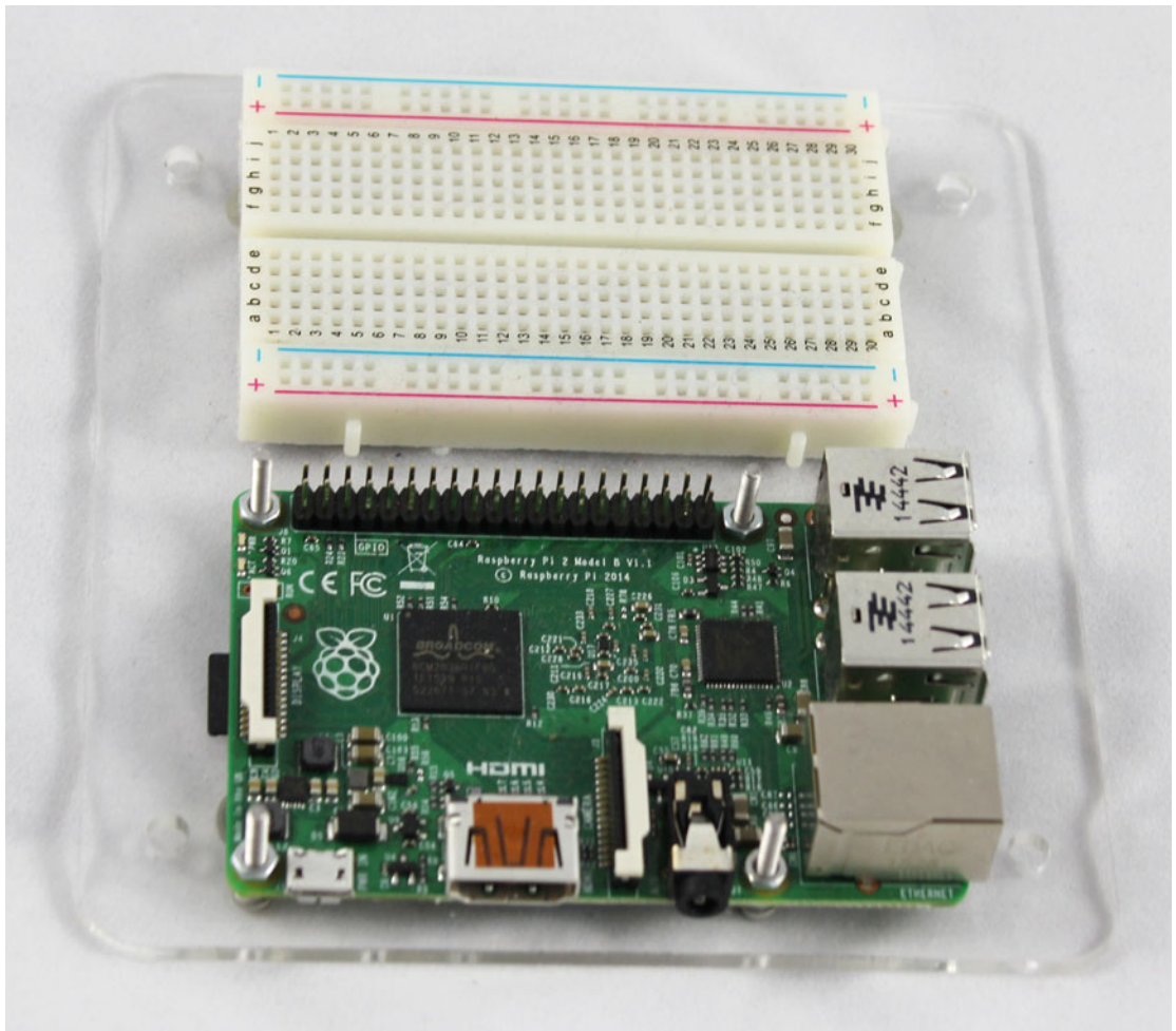
Figure 1-5. Raspberry Pi and a breadboard mounted together
