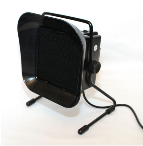
Figure 10-3. Bench-top fume disperser
