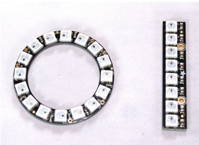
Figure 6-11. Adafruit NeoPixel ring and strip
