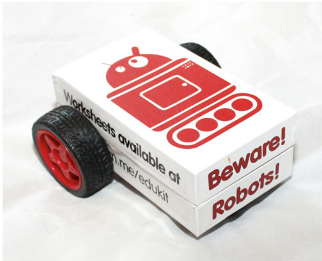
Figure 8-2. CamJam robot kit, with the box used as the robot chassis
