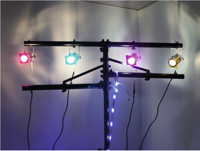
Figure 4-22. PAR 16 spotlights used as multi-colored disco lights
