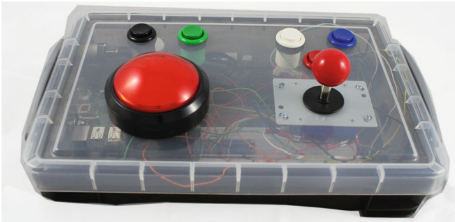
Figure 3-21. Enclosure with joystick for the arcade game
