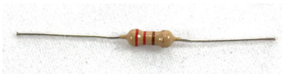
Figure 3-5. A 220 \Omega resistor
