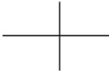
Figure 4-15. Circuit diagram representation of crossing and connecting wires
