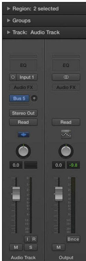
Figure 16-4: The inspector channel strips.
