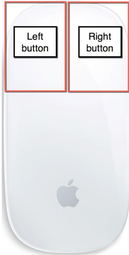
Figure 1-10. The top corners of the Apple mouse represent the left and right buttons
