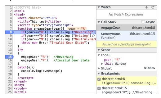
You can observe that the **Call Stack** window shows you how we arrived at line **8**. The **Scope** panel shows the **Local** scope where you can see the variables in the scope when the breakpoint was arrived at. You can also step into or step over the next function.
