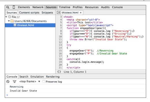
This is the view of the **Sources** panel. You can see the HTML and embedded JavaScript source in this panel. You can see the **Console** window as well. You can see that the file is executed and output is displayed in the **Console**.
