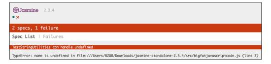
As you can see, the failure is displayed for this test case in a detailed error stack. Now, we go about fixing this. In your original JavaScript code, we can handle an undefined condition as follows:
