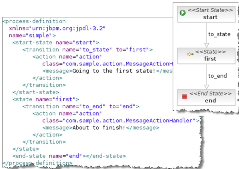
Figure 5.10 A jBPM sample process created automatically when a new process project is created
