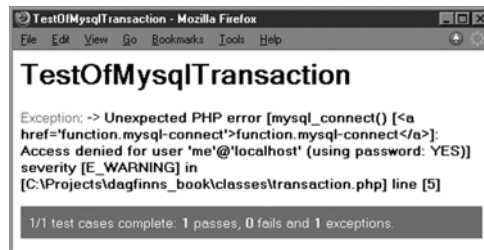
Figure 9.7 This time we're unable to get the MySQL connection, and the test case tells us what's wrong.
