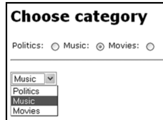
Figure 18.1 A plain drop-down menu is functionally equivalent to a set of radio buttons
