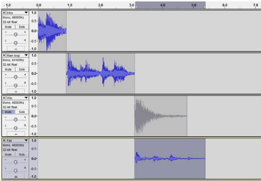
Figure 7-1. Horizontally queued music, without gaps, shown in Audacity. Note the muted “win” track.
