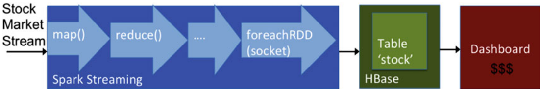
Figure 6-3. Stock market dashboard powered by Spark Streaming and HBase
