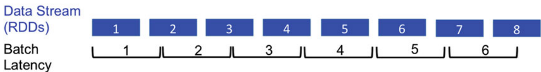
Figure 4-3. Mismatch between the input data rate and batch latency (or the set batch interval)
