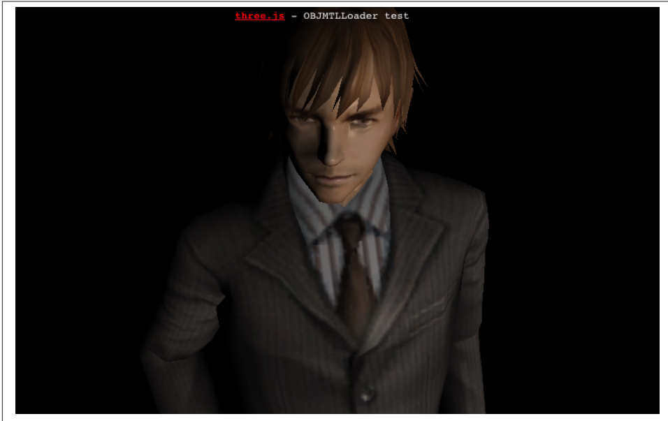
Figure 4-6. Mesh loaded from a file in Wavefront OBJ format
