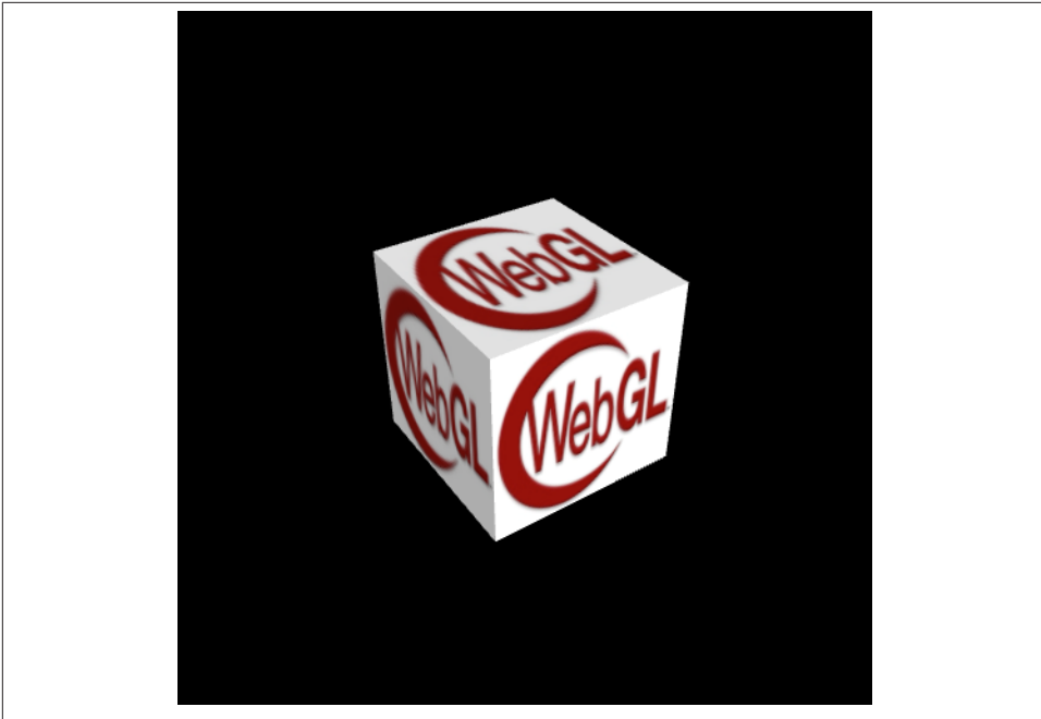
Figure 3-6. Three.js cube with lighting and Phong shading
