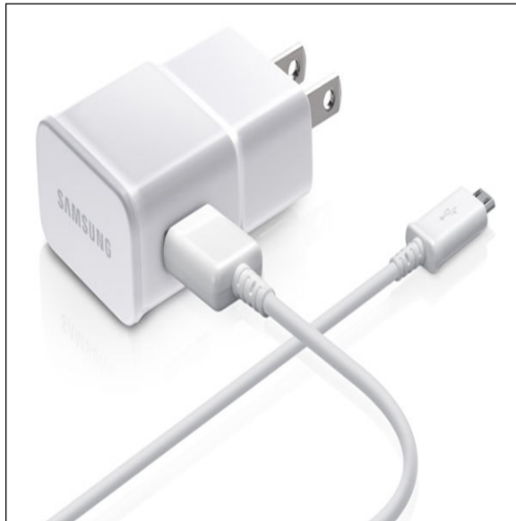
FIGURE 2-2: The transformer and USB cable for charging your phone.
