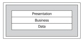
Within the tenets of client-server architecture, the single tier application can share the data layer in a multi-user environment and achieve the client-server capabilities. The limitations of 1-tier application in client-server architecture are as follows:
