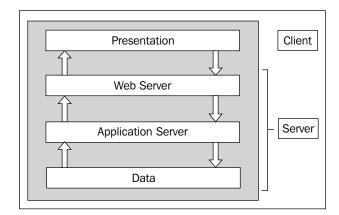
In a typical web-based solution, the client will have access to the business through a browser. The browser in turn will call the business logic in the web-server. The web server will subsequently transfer the calls to the application server, which effectively sends the request to the data layer.
