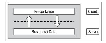
As the business logic was independent of the presentation logic, it enabled different forms of GUI to connect to a particular business process. The GUI would be served as a simple HTML application, or it could be any form of complex presentation logic.
