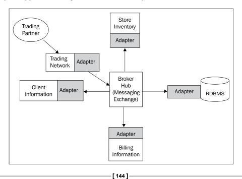
The preceding image depicts integration between various systems in an enterprise. Now, we can see that the systems, which were hitherto monolithic, can communicate with each other. Also, external systems, say trading partners, communicate to the message broker using 'Trading Network' setups and adapters.
