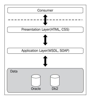
Shown here is a typical architecture for a database driven, web-based solution. It provides us with a high-level overview of the entire system. The consumer only has a view of the 'presentation layer' and other layers are tightly encapsulated. Each layer would have its own characteristics as well as its own architecture.
