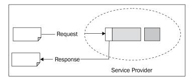
• **The Service Consumer**: The consumer would send out a message to the provider in order to access the service. This is the requester. It would either be done directly by a service-to-service call or through the directory services. Services required for processing are identified by their service descriptions.
