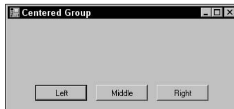
Figure 2-17: Controls with Anchor set to Bottom remain centered as a group.
