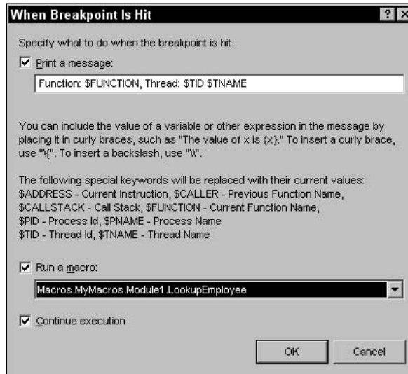
Figure 1-35: The When Breakpoint Is Hit Condition dialog lets you determine what actions Visual Basic takes when the breakpoint is activated.
