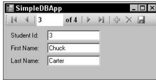
Figure 11-14: Drag and drop table columns onto a form to create a record-oriented view instead of a grid.
