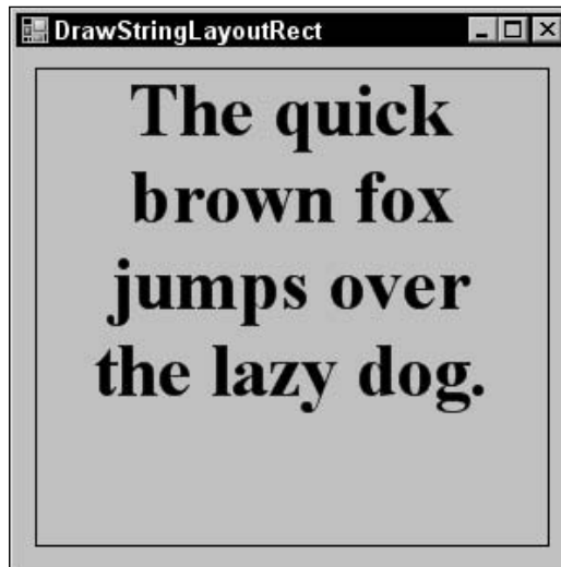
Figure 21-3: The DrawString method can use a layout rectangle and a StringFormat object to format text.
