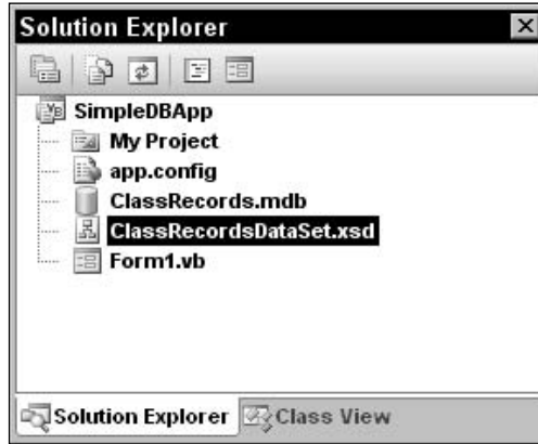
Figure 11-9: The Data Source Configuration Wizard adds a database and schema to Solution Explorer.
