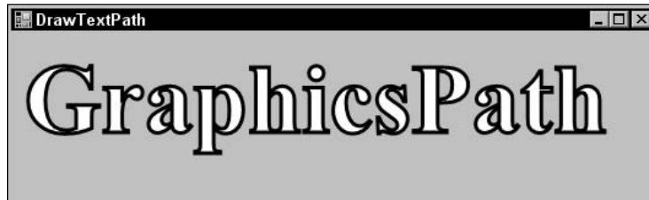
Figure 19-11: The DrawPath method draws the outline defined by a GraphicsPath object.
