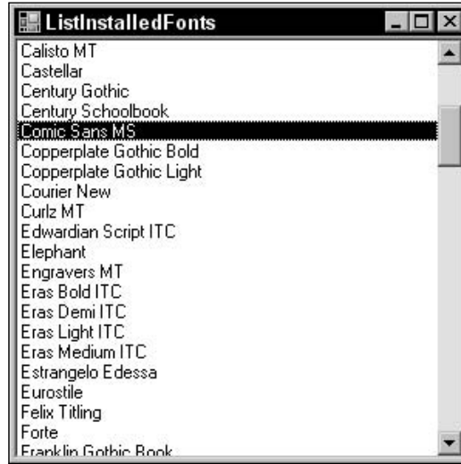
Figure 19-5: An InstalledFontCollection object provides access to an array of FontFamily objects representing the fonts installed on the system.
