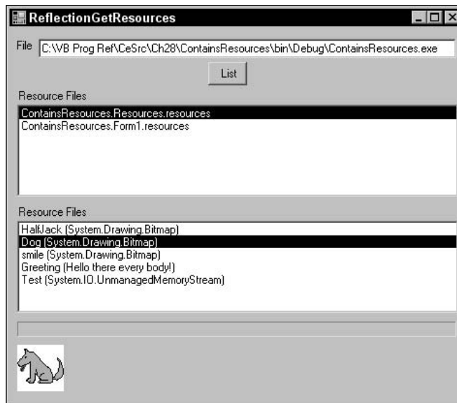
Figure 28-4: This application uses reflection to display another application's resources.
