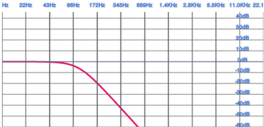
Figure 6-1. Frequency response graph for a low-pass filter
