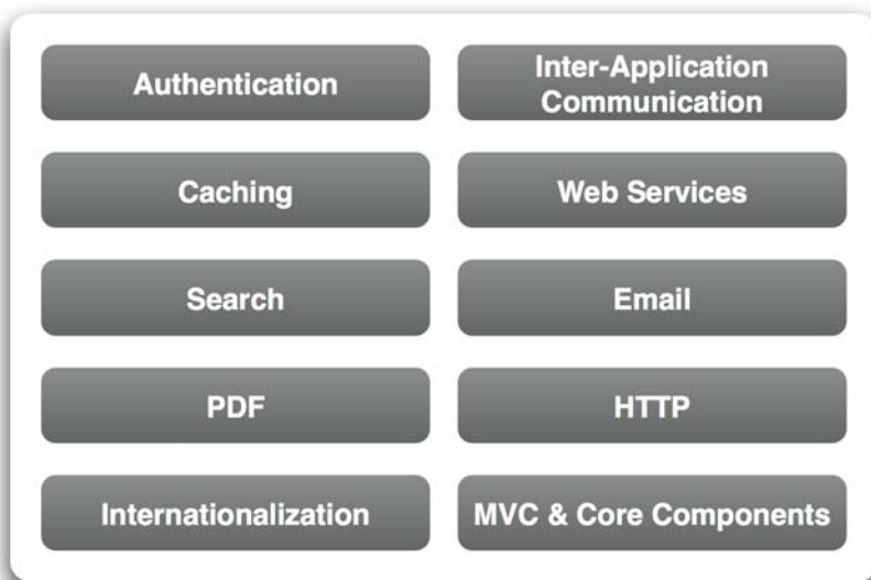
Figure 1.3: The Zend Framework can be divided into ten main modules
