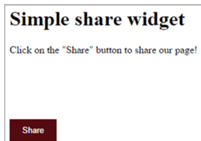
Figure 5.1a The presence of the hidden class is toggled whenever the user clicks the button, causing the box to be shown or hidden. In its initial state the box is hidden.
