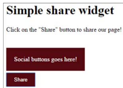
Figure 5.1b When the Share button is clicked, it toggles the hidden class. This figure shows the box when displayed.
