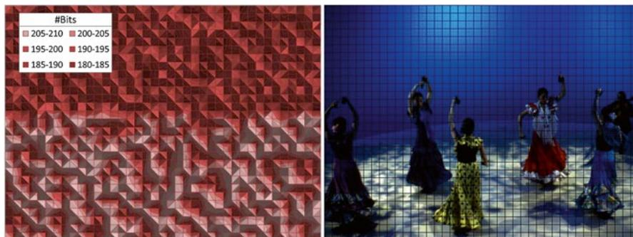
Fig. 4.12 Basic unit-level bitrate distribution (Flamenco2, QP=32)
