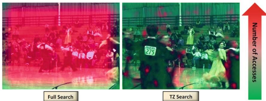
Fig. B.5 Output example: reference frame access index considering two block matching algorithms: full search and TZ search
